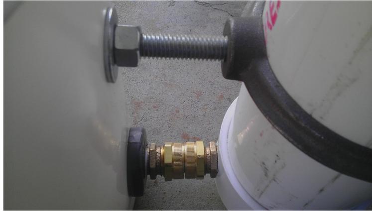
4. Align garden hose adapter to the side of the 5gal bucket while BFA and bucket are upright and on a flat surface. Mark center of hole. Use handle to find center placement of BFA on bucket.
